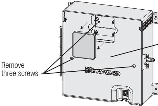
Pull the small cover away from the panel by grasping it with your hand (no tools required). Then, remove the 3 screws and pull the plastic deadfront panel away from the enclosure.
