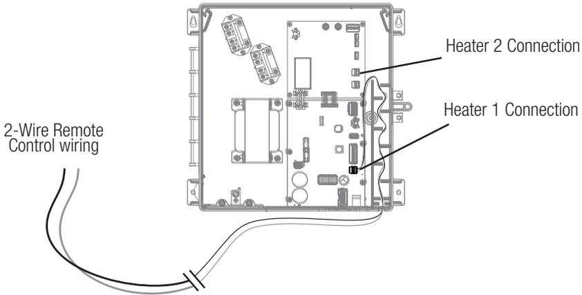
1. Wire heater to 120/240V power source per the instructions in the heater manual. The AQR S3 Omni does NOT control the power going to the heater.
