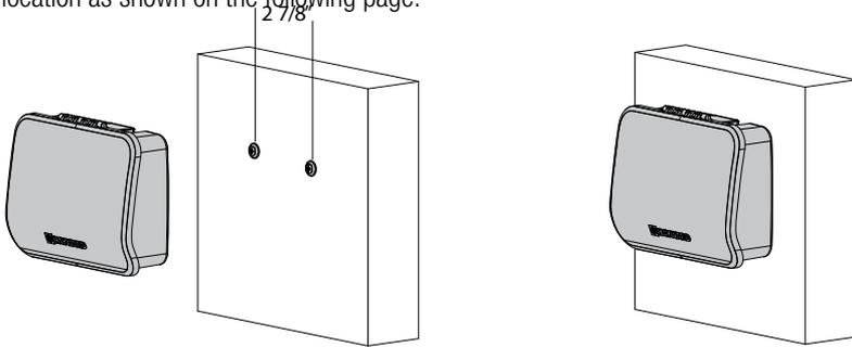
Tighten until the bottom of the screw heads are 1/8" off the mounting surface. Position the Controller cutouts over the screw and slide the unit downward. You may have to tighten or loosen the screws slightly to fully engage the screw heads to get a snug fit.
