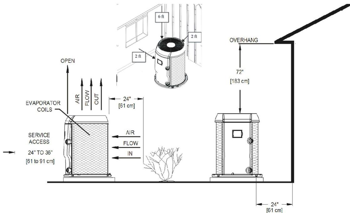
**NOTE:** The clearances shown above are for best practice and we encourage the use of the best practice clearances when the space is available. Exceptions can be made where the size of the lot or the configuration of fences, walls or other associated structures do not allow for the best practice clearances. Testing has shown this heat pump can be installed as close as 6" (to coil) from a restriction (Wall, Fence, etc.).
