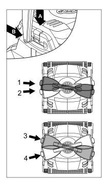
Change diagonal handle position for water line sideway movement. To adjust the handle angle:
